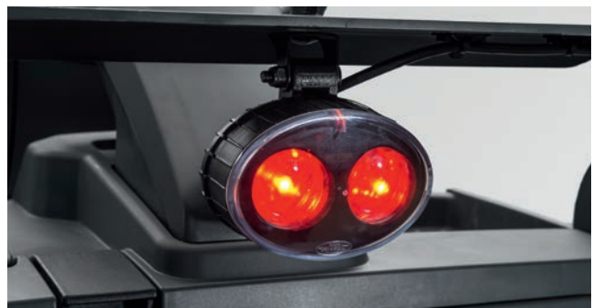
Floor-Spot for safe manoeuvring
