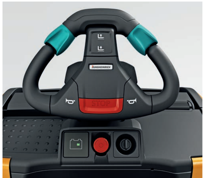
JetPilot: The height-adjustable multifunctional steering wheel
