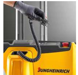
Easy intermediate charging thanks to on-board charger.
