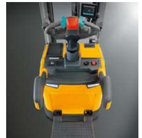
Plenty of room for movement for the operator as well: The stand-on platform of the ERC 216z.
