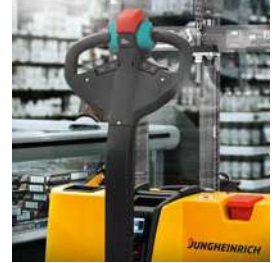
Easy and safe to manoeuvre: The safety control handle of pedestrian trucks.
