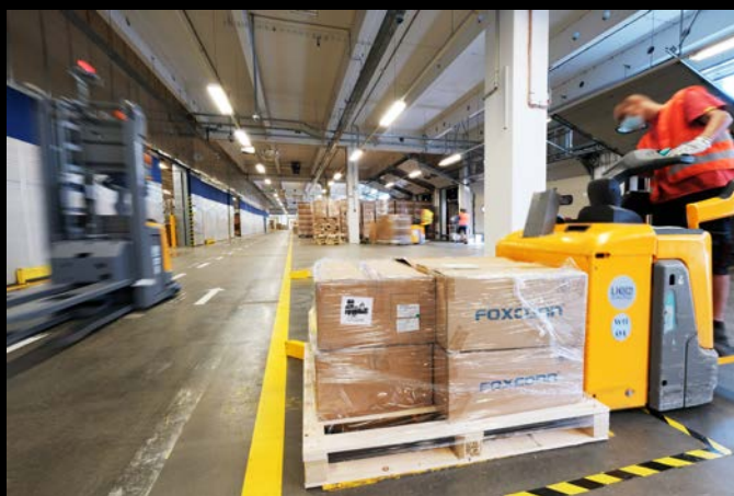
The Jungheinrich ERC 215a Automated Guided Vehicle works at FOXCONN in mixed operation among the warehouse's other technology and workers.
