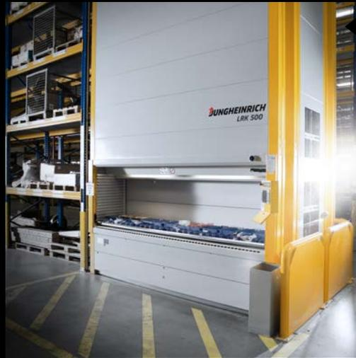
Compact storage of goods in vertical lift and paternoster racking with direct integration into the Jungheinrich WMS.
