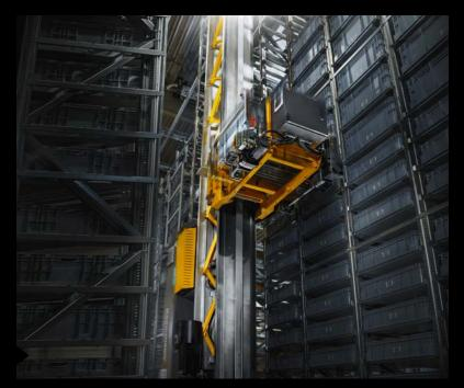
Automatic miniload warehouses and the corresponding stacker cranes are used in high-performance environments and are controlled via the Stacker crane module in the Jungheinrich WMS. With the use of stacker cranes, the putaway of goods from the workplaces as well as the retrieval of goods to the workplaces take place automatically. This enables you to enjoy accelerated processes and a reduced error rate.
