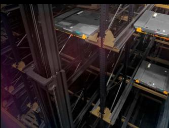
Double or multi-depth storage, e.g. in channel warehouses, drive-through storage racking, push-back or drive-in racking, can also be mapped in the Jungheinrich WMS. When storing or retrieving goods in multi-depth areas, the Jungheinrich pallet shuttle can also be fully integrated and controlled via the Jungheinrich WMS.
