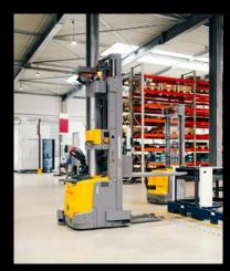
The AGVs deliver the materials directly to the machines and workplaces which so-called docking stations. They use sensors to detect the load carriers and report receipt of the material to TruTops Fab.
