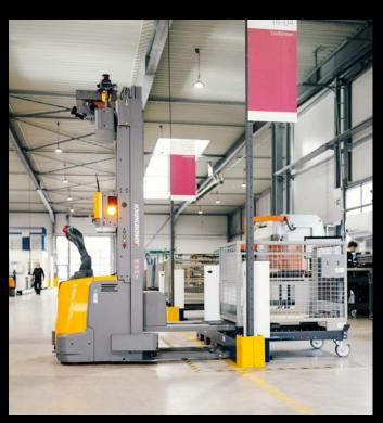
An ECR 213a AGV is in operation at DAX. It handles 22 transports per hour, automatically transferring around 80 percent of the parts through the production process at DAX.
