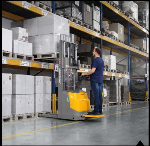
With a lift height of up to 4,700 mm, the ERC 1i makes storage and retrieval at higher racking levels simple.
