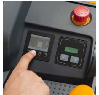
All key parameters always in clear view, such as battery charge level and operating hours.
