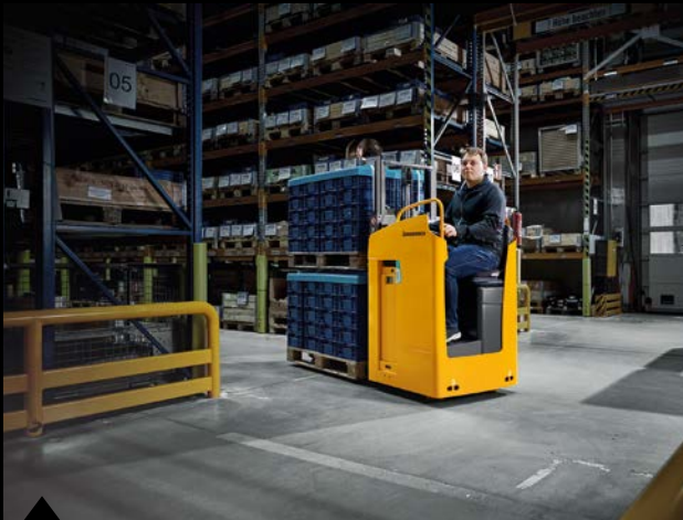
The ergonomic sideways-seated position gives the operator excellent visibility, even during frequent direction changes.
