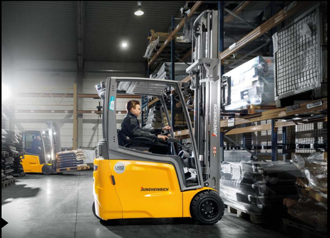
The powerful hydraulics enable the EFG 216k to achieve high lift speeds.
