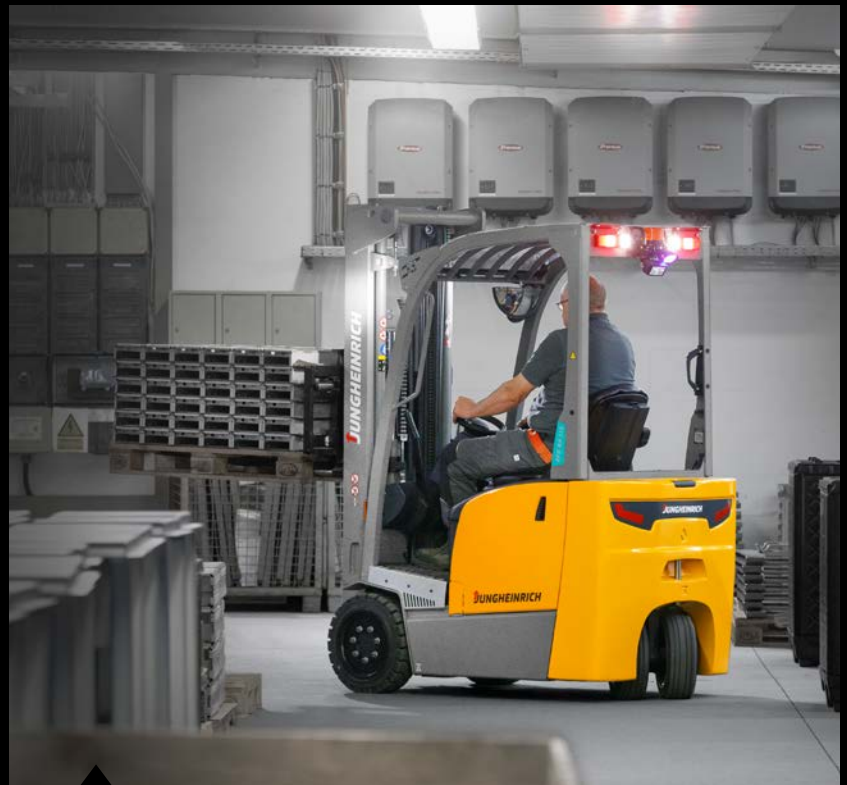
Available as standard, curveCONTROL automatically reduces cornering speed.
