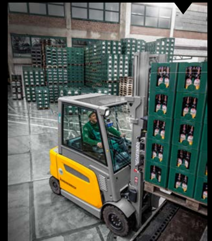
The combination of slimline B-pillar design and panoramic roof guarantees optimum visibility.
