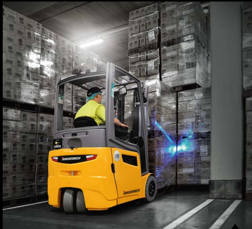
The Floor-Spot projects a blue light onto the floor in front of the truck, which alerts employees to the approaching industrial truck.
