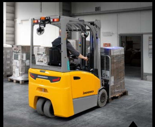
The manoeuvrable three-wheel counterbalance forklift truck boasts a compact design and is particularly impressive at delivering flexible transport within confined warehouse environments.
