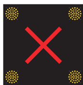
Tunnel Lane Closed
