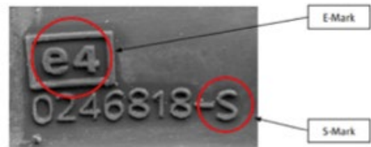
Figure 2: E-Mark and S-Mark on tyre sidewall
