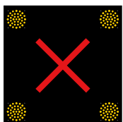
Tunnel Lane Closed
