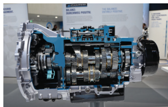
Example of cutaway synchromesh gearbox.
