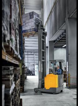
Lithium-ion stackers are specially designed for multi-shift operation and can easily be booster charged during breaks.
