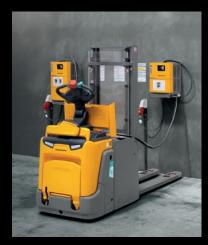
Lithium-ion batteries enable rapid and booster charging during breaks and downtime for maximum truck availability.
