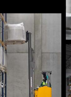
Agile and economical: the ETV 216i reach truck with lithium-ion technology is ideally suited for efficient storing and removal at lift heights of up to 13 metres.
