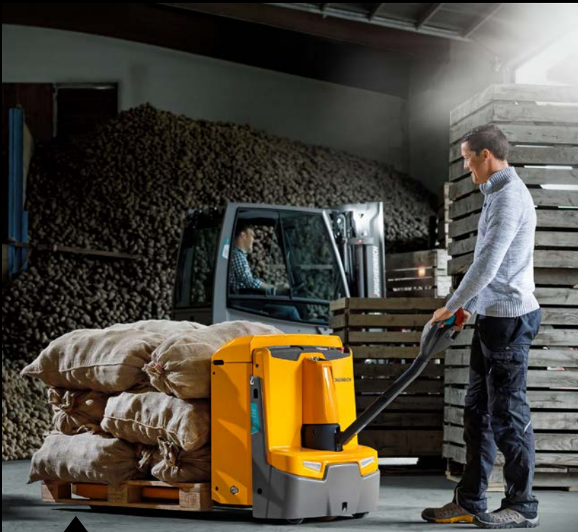
The EJE 1 series boasts integrated support wheels linked via a torsion bar for outstanding driving stability.
