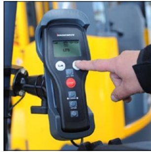
UPC operation via hand-held radio terminal
