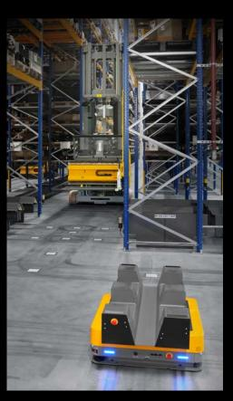
Efficient, scalable and flexible. At the heart of this innovative intralogistics solution is the unique combination of 15 autonomous mobile robots arculee S and 8 EKX 516ka mobile robots for automated VNA storage.
