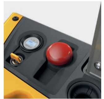
The EJC M: All important control instruments are arranged centrally: battery discharge indicator, hourmeter, emergency disconnect and key.
