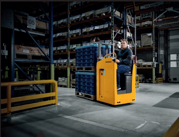
The ergonomic sideways-seated position always gives the operator the best view, even when changing direction frequently.
