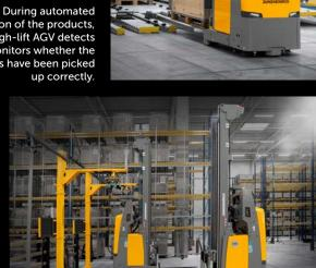
24/7 availability guaranteed: The AGV uses times without transport orders to temporarily charge its lithium-ion battery at an automatic charging station.
