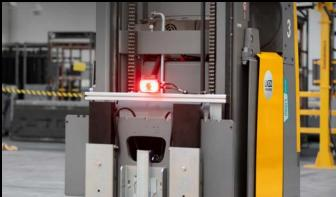
The products are identified using a QR code scanner before the Logistics Interface coordinates storage in coordination with the customer's own WMS.
