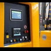
The 7-inch display with touch function provides a quick overview of the current battery charge level and other important storage process data.
