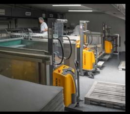
Always at the optimal handle height: when used as a working platform with materials handling equipment, the HC 110 electric stacker truck provides back boxes for production.
