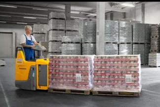
Thanks to its long forks, the ERE 225i electric pallet truck can easily transport two pallets at the same time.
