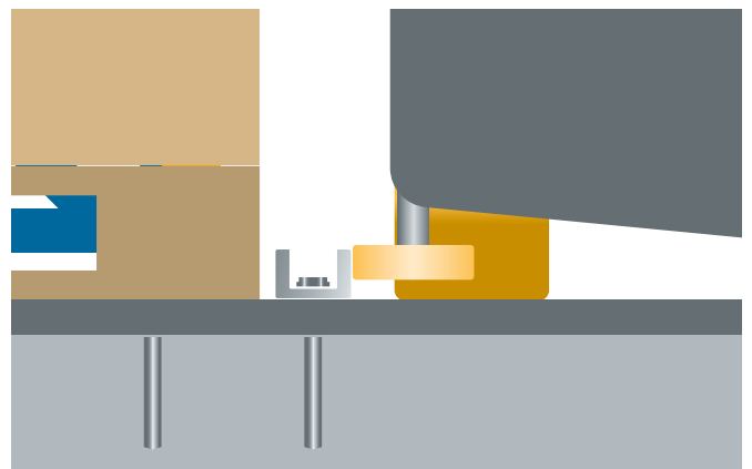
Fig. 6 Low guide rail, e.g. U profile 65/42/6.
