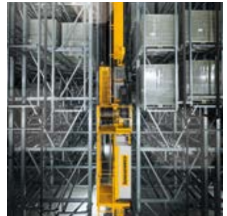
Stacker crane for pallets: speed and precision during storage and retrieval process.
