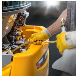
Regular replacement of the hydraulic oil significantly reduces wear. This avoids unnecessary repairs.
