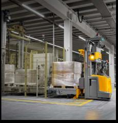
Pallets are wrapped in stretch film to ensure the safe transport of goods. The Jungheinrich Logistics Interface uses a specially designed interface solution, the AGV/AMR Connector, to enable a continuous, automated material flow between the pallet stretchers and the mobile robots.
