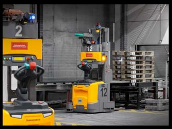
The mobile robots control pick-up and drop-off points. In addition to finding suitable interfaces, the narrow travel paths in the existing structures were a challenge for automation.
