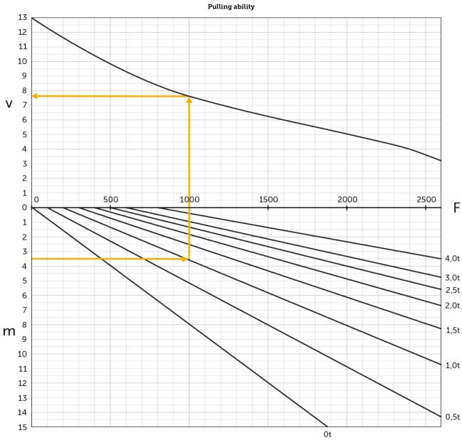
v=speed [km/h], m=incline [%], F=drawbar pull [N]
