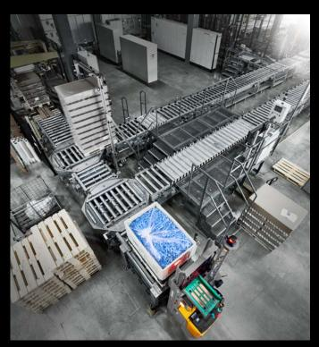
Full speed ahead: The AGV transports the required raw materials to the production machines quickly and effortlessly.
