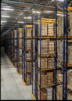
The warehouse features 36 aisles with a width of over three metres and is equipped with conventional pallet racking up to a height of 10.4 metres.
