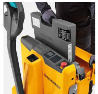
The battery can be removed and replaced in just a few steps.
