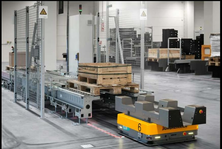
Efficient, scalable and flexible. At the heart of this innovative intralogistics solution is the unique combination of 15 autonomous mobile robots arculee S and 8 EKX 516ka mobile robots for automated VNA storage.
