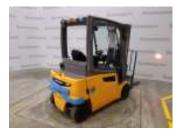
EFG 316 Li SP GE 115 FN545854 2017 1,600 kg Load capacity: 1,600 kg 4,400 mm Lifting height: 4,400 mm Mast type: Three-stage free lift 51 V / 480 Ah 48 V / 55 A Charger: 48 V / 150 A £14,393 Price: £14,608
