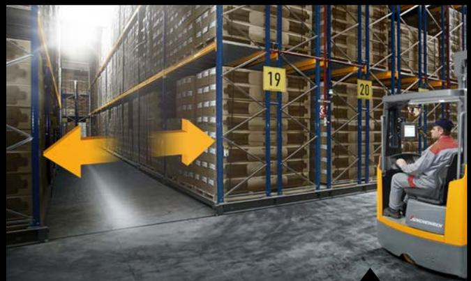
Greater efficiency: with mobile racking with WMS connection, the working aisle is already opening on approach.
