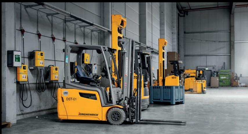
Lithium-ion stackers are specially designed for multi-shift operation and can easily be booster charged during breaks.
