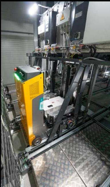
For increased productivity, the shuttles can be serviced individually outside the system while the remaining shuttles continue operating.
