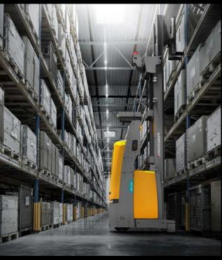
Future-proof warehouse solution from Jungheinrich: utilisation of an automated truck with a lithium-ion battery.
