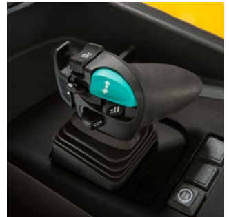
One-handed control of all functions thanks to multiPILOT.
