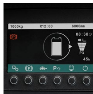
Clear display with travel direction display for the five different steering modes.
