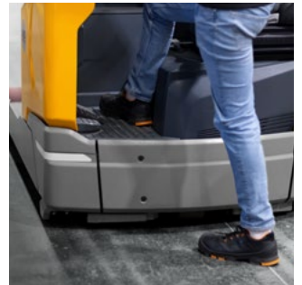
Ergonomically designed: the low step height facilitates frequent entry and exit.
