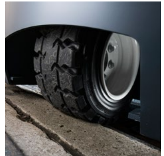
The high ground clearance guarantees comfortable travel even over thresholds without bottoming out.
