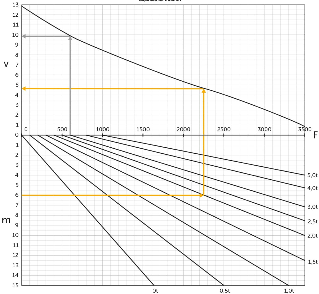
v = vitesse [km/h], m = pente [%], F = force de traction [N]
