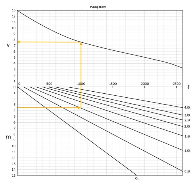
v=speed [km/h], m=incline [%], F=drawbar pull [N]
