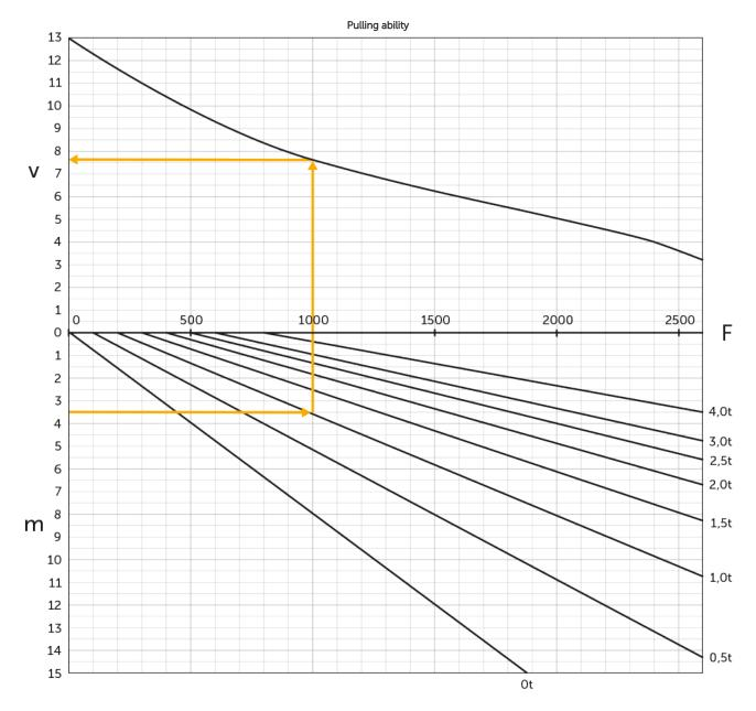
v=speed [km/h], m=incline [%], F=drawbar pull [N]
