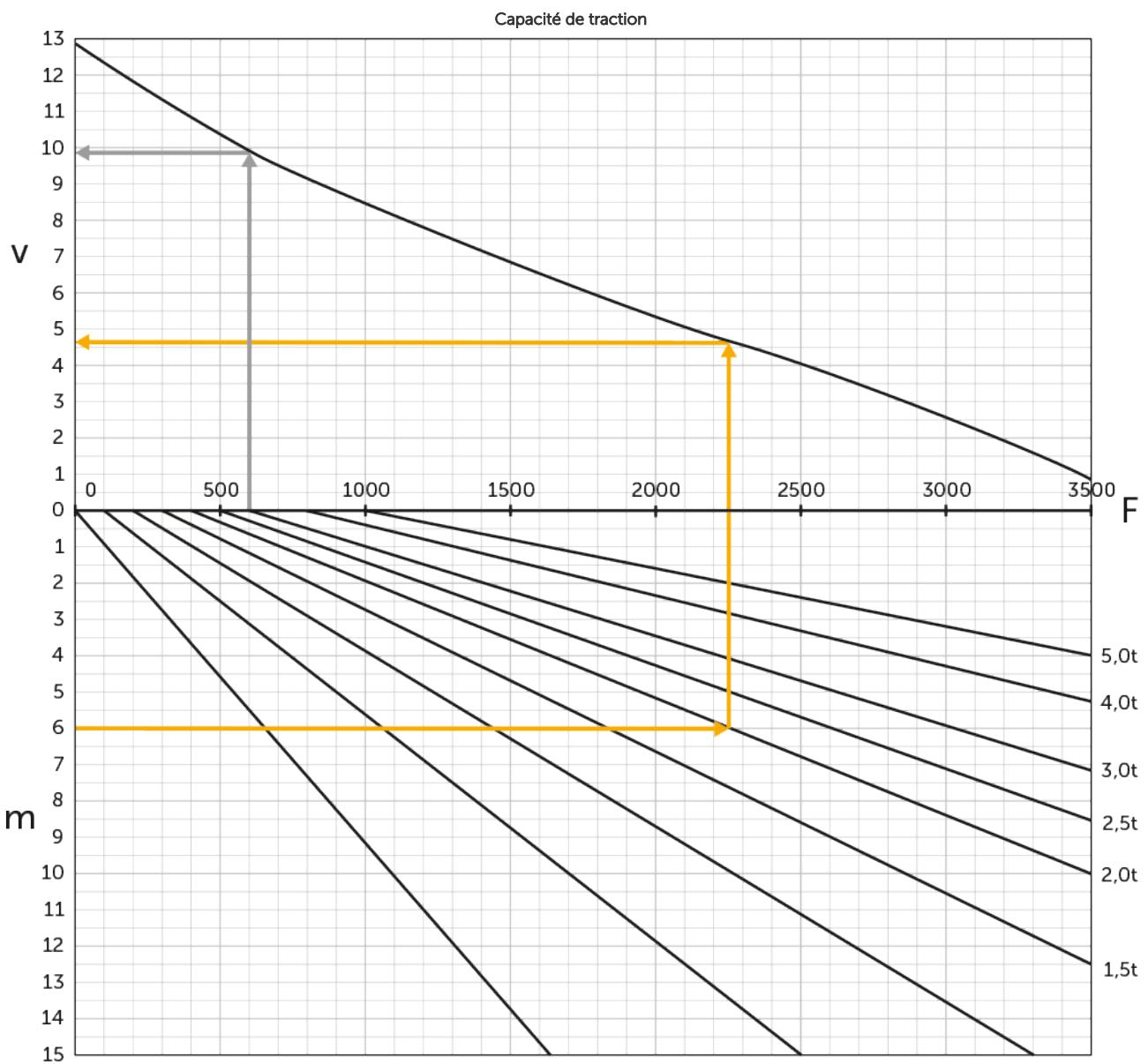
$v$  = vitesse [km/h],  $m$  = montée [%],  $F$  = force de traction [N]
