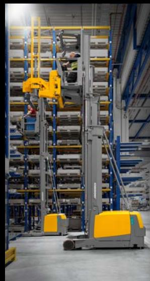
In narrow aisles with single-bay racking, forklift trucks handle the ergonomic order picking of the various items.
