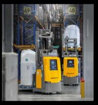
Perfect teamwork: the mobile robots hand over the pallets to the manual narrow-aisle trucks for further transport.
