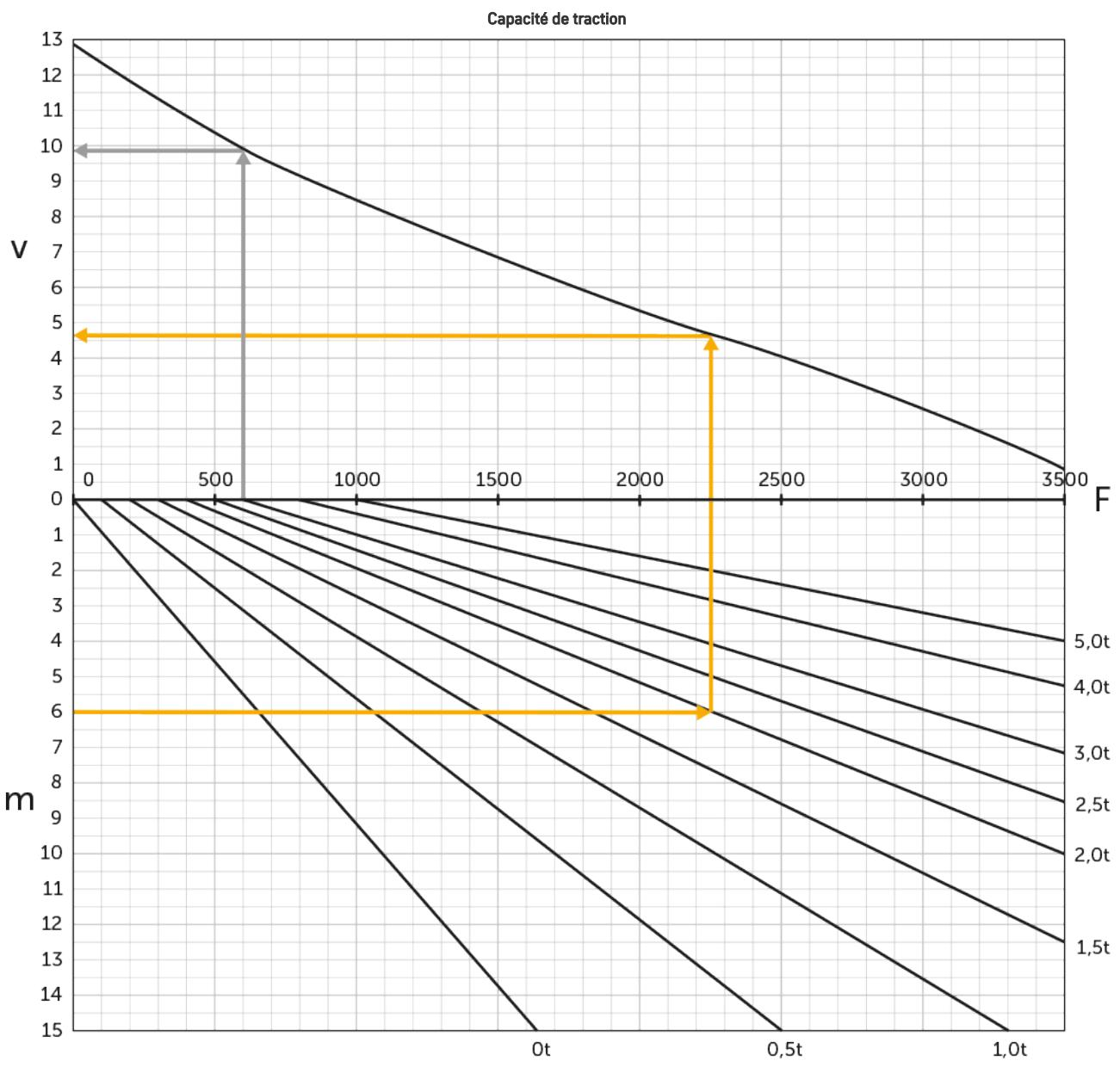
$v$  = vitesse [km/h],  $m$  = montée [%],  $F$  = force de traction [N]
