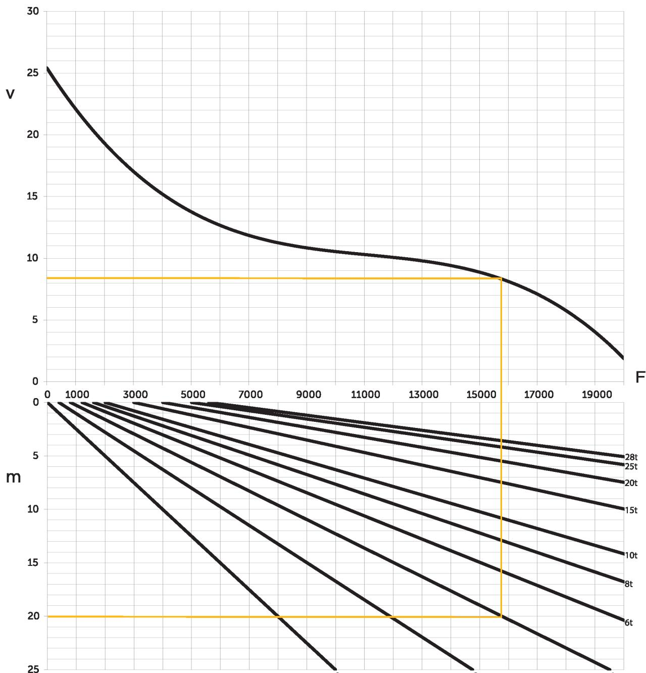
$v$ =speed [km/h],  $m$ =incline [%],  $F$ =drawbar pull [N]
