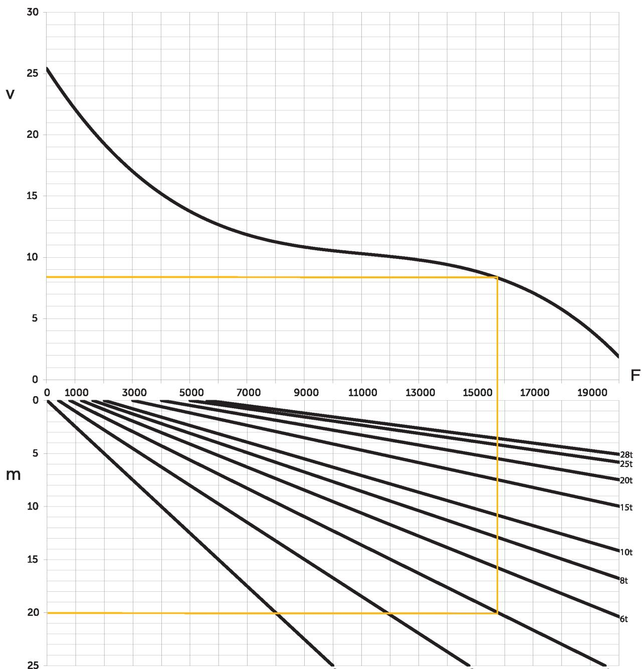
$v$  = vitesse [km/h],  $m$  = montée [%],  $F$  = force de traction [N]
