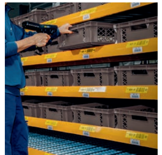
The FIFO principle of the carton live storage makes it possible to monitor batches and best before dates.
