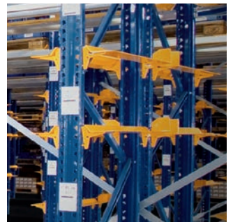
Single-bay racking: angle profiles arranged in the depth direction take on the beam function, permitting extra space height wise.
