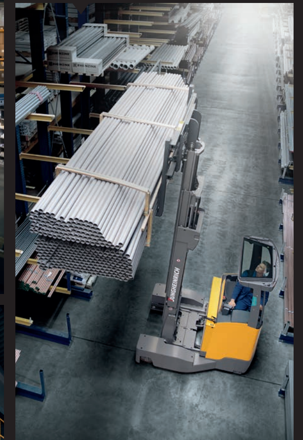
Cantilever racking is ideal for storing long goods. It continually adapts to individual requirements.
