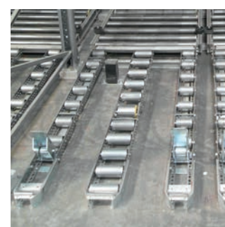
The three-piece design of the floor coasting with a run-out height of approx. 66 mm ensures gentle pallet removal.
