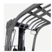
Arched overhead guard for optimal visibility typical of the BB and BC series.
