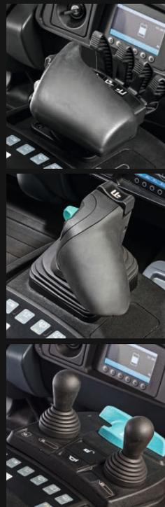
**soloPILOT:** All hydraulic functions, travel direction selection and horn in a single lever. Control of all functions with millimetre precision.
