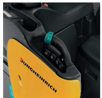
The multi-function lever offers full control over all lift and travel functions, even without changing your grip.
