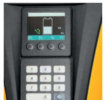
EMC 110: 2-inch truck display including discharge indicator and hourmeter (optional).
