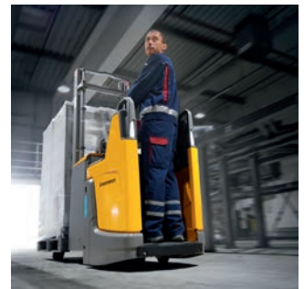
Spacious stand-on platform for maximum ergonomics and operator safety. Optionally with foot protection sensor.
