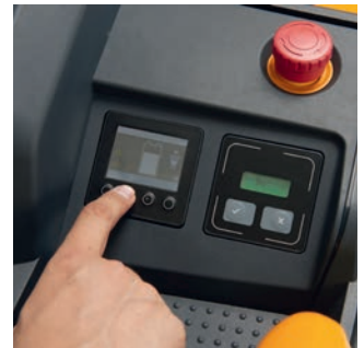
All important parameters always in view, e.g. charge state or operating hours.
